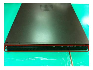
Start by removing the front plate.
